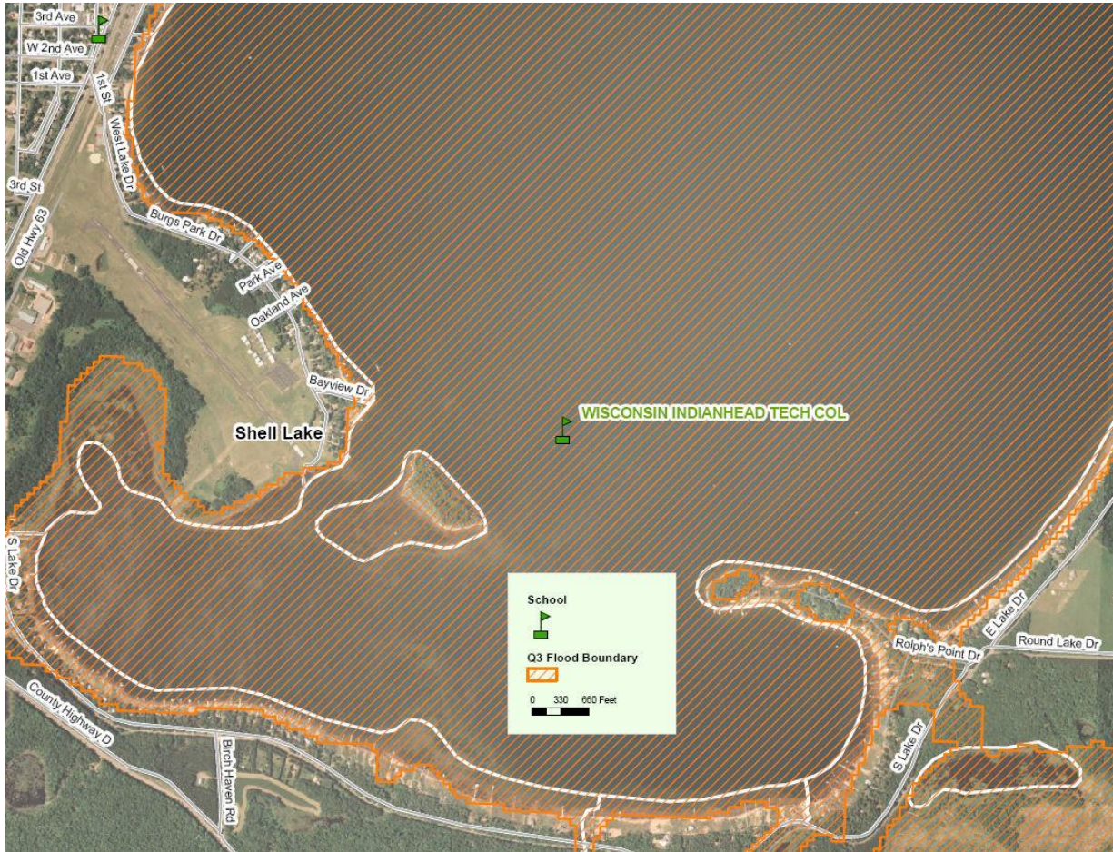
Figure 4: 100-Year Flood Boundary Overlaid with Essential Facilities
